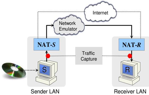
**Figure 1 – The testbed for the experiments**
