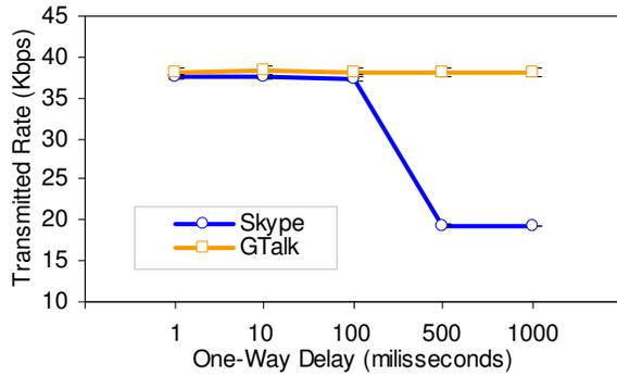
Figure 6 –Throughput for different delays
