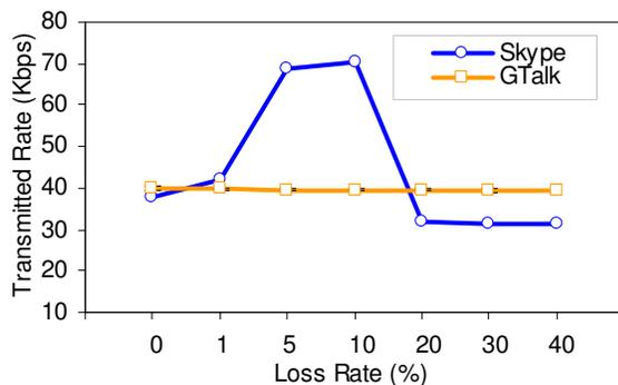
Figure 8 – Throughput for different loss rates
